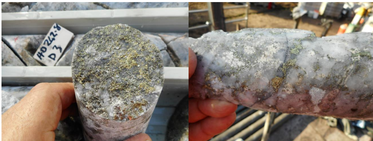
Figure 2 Briggs BD019-003, Chalcopyrite (Copper) Mineralisation in Quartz Zone
