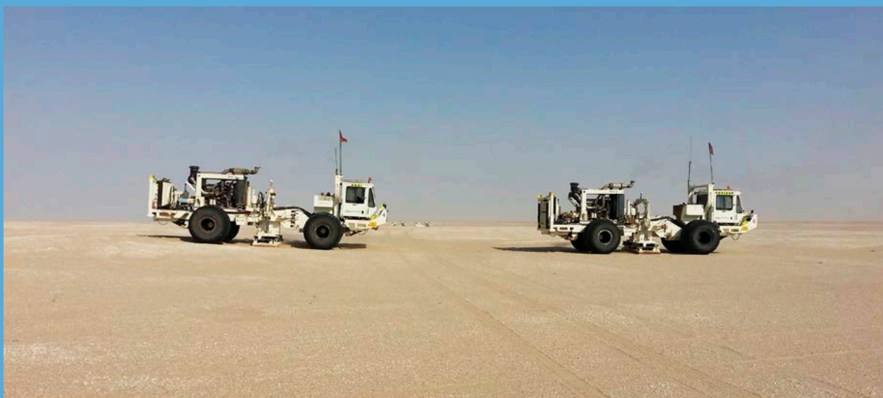
Vibrator trucks at Blocks 3&4
