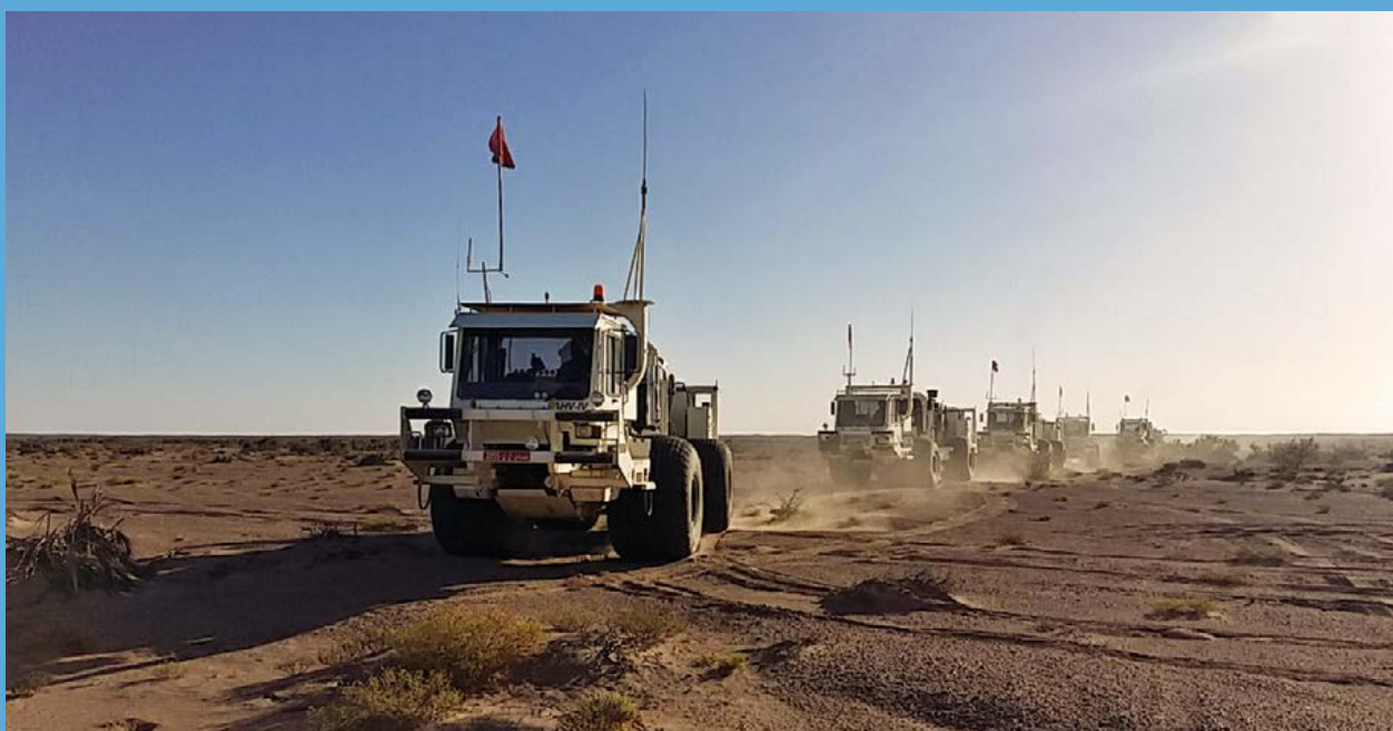
Vibrator trucks at Blocks 3&4
