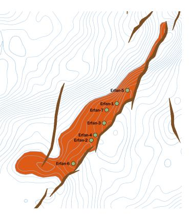
The Erfan oil field is a single structure producing from the Khufai carbonate formation, at depths ranging from 1,700 to 2,400 metres, in the same producing formation as in neighbouring Saiwan East field.
