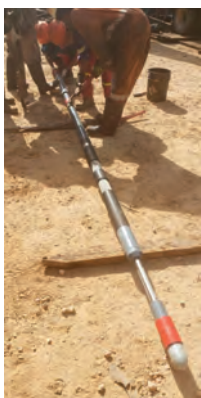
Downhole plug used to isolate the reservoir zone for CO2 injection
