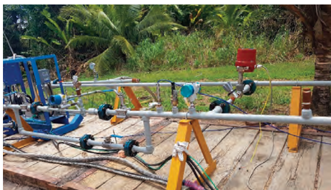
Part of CO2 delivery system constructed at Inniss-Trinity
