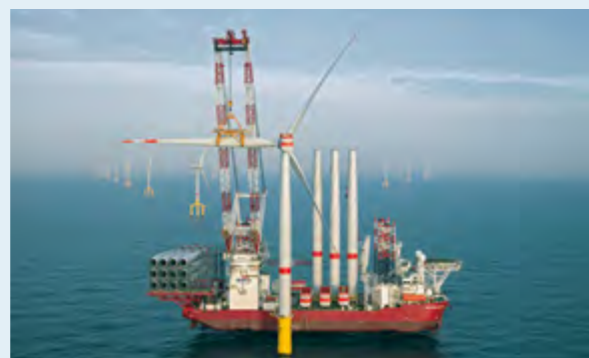
One of the world's largest self-elevating platform vessels owned and operated by Seajacks
