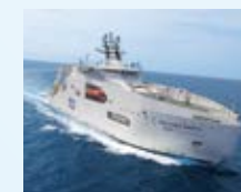
▶ Power-cable laying Operation of cable-laying ships capable of laying power transmission lines
