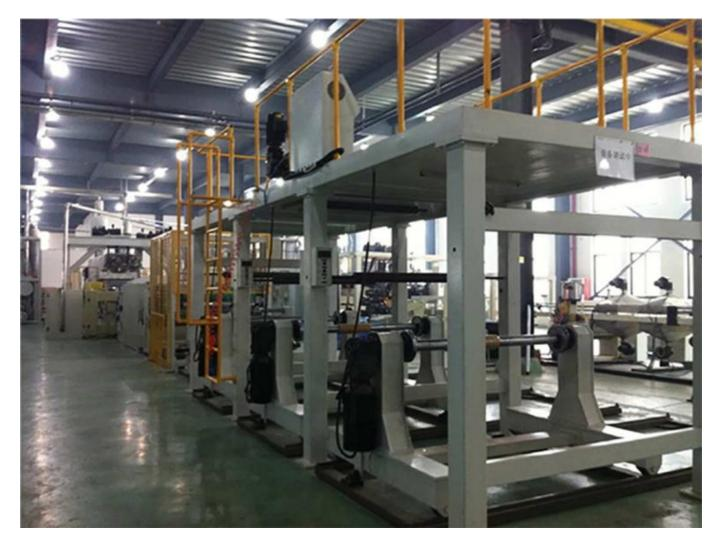
Four-Layer Co-Extruded Sheet Machine in our Sanmen factory.
