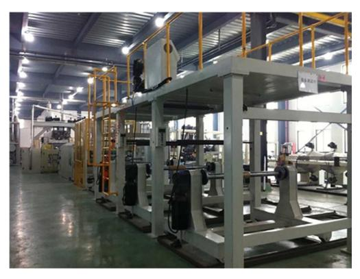
Four-Layer Co-Extruded Sheet Machine in our Sanmen factory.
