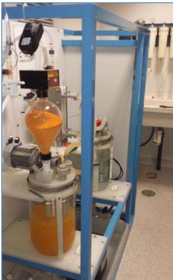
Figure 4 - Initial Vanadium dosing of Acid
