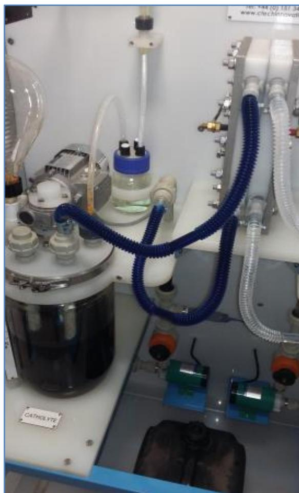
Figure 5 - Balanced Vanadium electrolyte
