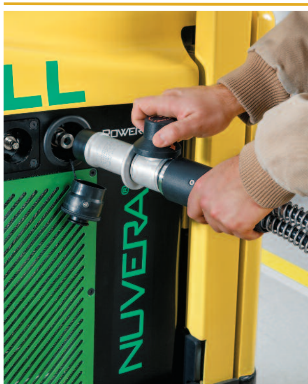
A Hyster® fuel cell-powered lift truck with a Nuvera PowerEdge® unit refuels at a hydrogen dispenser.
