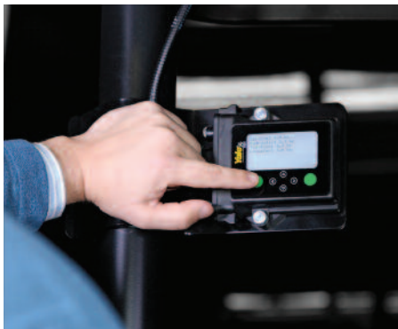
A Yale Vision telematics solution shown mounted on a Yale® lift truck. The Yale Vision tracks over five usage meters, including impact sensing, access control and preventive maintenance and, ultimately, helps promote both operator safety and increased productivity.
