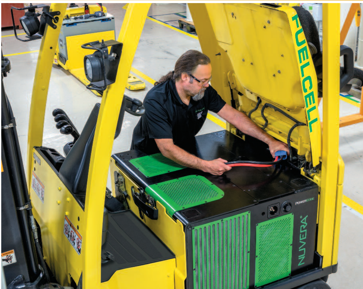
An employee installs a PowerEdge® battery-box replacement in a Hyster® 4-wheel electric truck.
