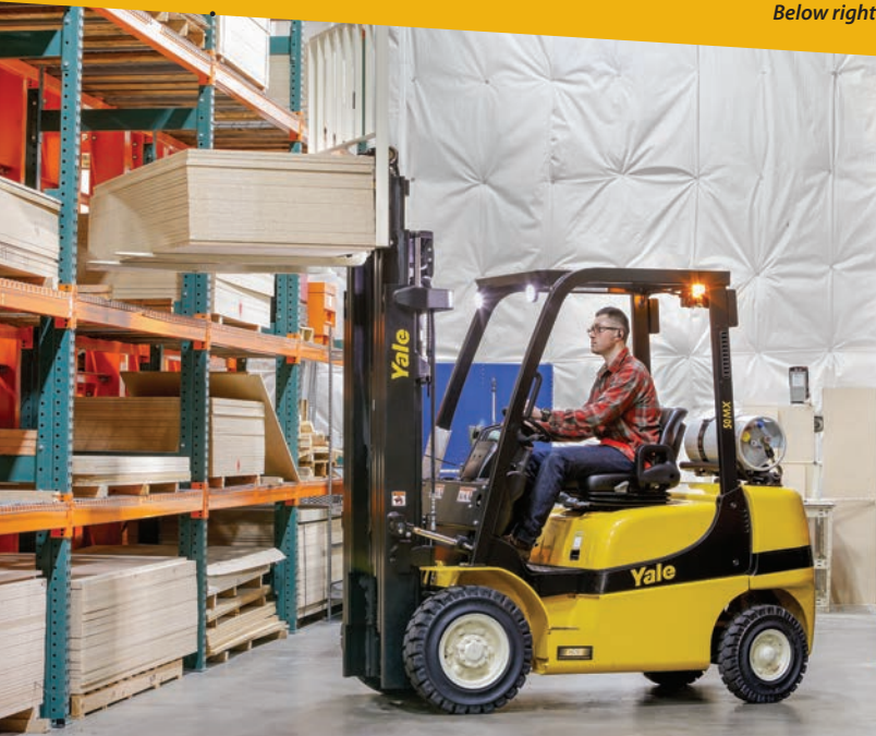
Below left: The new Yale® 50MX standard pneumatic-tire, internal combustion engine lift truck has a basic lifting capacity of 5,000 pounds and is designed to fit into almost any application or industry needing a hard-working forklift.
