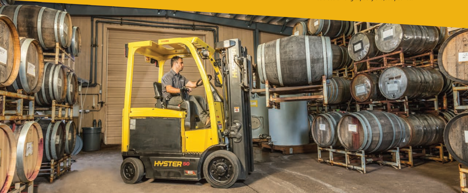
The Hyster® E50XN Next Gen 4-wheel, cushion-tire, counterbalanced electric truck, shown moving barrels at a winery, has a basic lifting capacity of 5,000 pounds.
