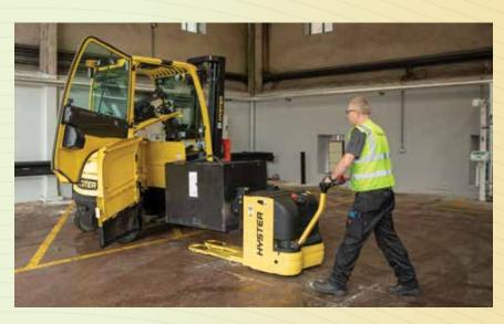
◆ An electric Hyster® J3.5XN counterbalanced truck equipped with a side-battery exchange option, used in a beverage application, is having its battery quickly changed with the assistance of a Hyster® powered battery-exchange stacker.
