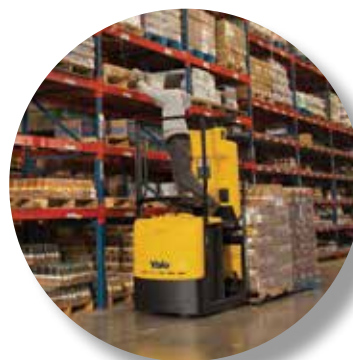
Left: A Yale® MO5.0T electric robotic tow tractor equipped with “Driven by Balyo” technology can tow up to 10,000 pounds and autonomously navigate through warehouse environments. ▲ Right: A Yale® second-level order picker lift truck, being used in a food distribution warehouse, allows access to an increased number of SKUs.
