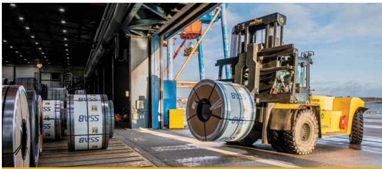
The Hyster® Big Truck range is built for demanding applications with heavy loads. A Hyster 32-12 Big Truck, with a lifting capacity of 32 tons, utilizes a side-shift fork positioner to store steel coils on a dock at a shipping port in Sweden.
