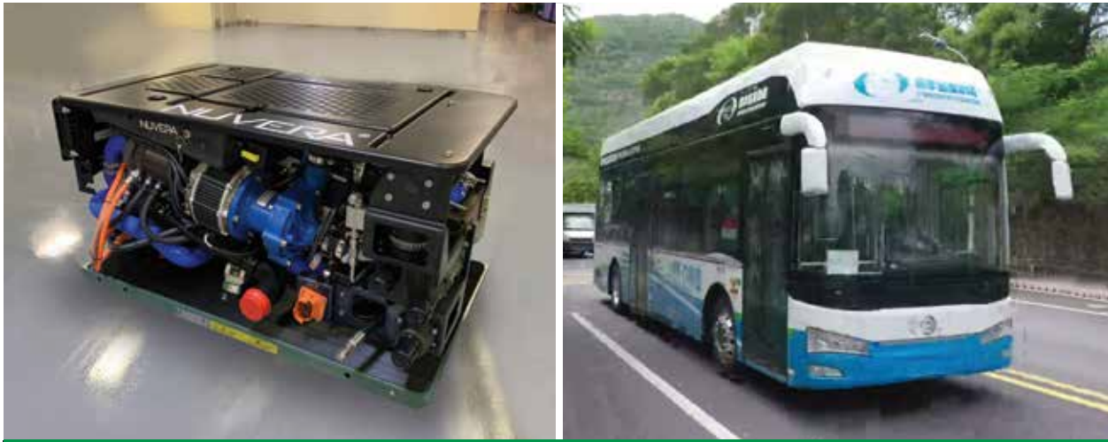
Left: The new Nuvera® 45kW engine that is being used in the electrified Big Truck for the Port of Los Angeles. ▲ Right: The same Nuvera® 45kW engine will be used in new heavy-duty applications, including, as shown, by a bus in China going through testing of this engine for an Asian customer.
