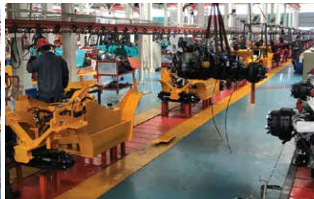
Left: The recently introduced Hyster® 3.0 UT low-intensity, pneumatic-tire lift truck, with capacity up to 3.0 tons, is shown moving crates in a warehouse in Turkey. ▲ Right: The Hyster-Yale Maximal assembly line in Fuyang, China, which uses Hyster-Yale's demand-flow technology manufacturing process, assembles low-intensity, internal-combustion engine lift trucks for supply both locally and globally.
