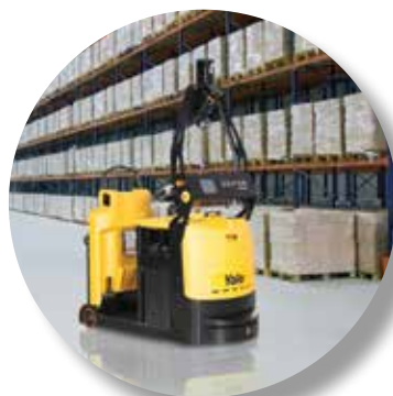
Left: A Yale® MO5.0T electric robotic tow tractor equipped with “Driven by Balyo” technology can tow up to 10,000 pounds and autonomously navigate through warehouse environments. ▲ Right: A Yale® second-level order picker lift truck, being used in a food distribution warehouse, allows access to an increased number of SKUs.
