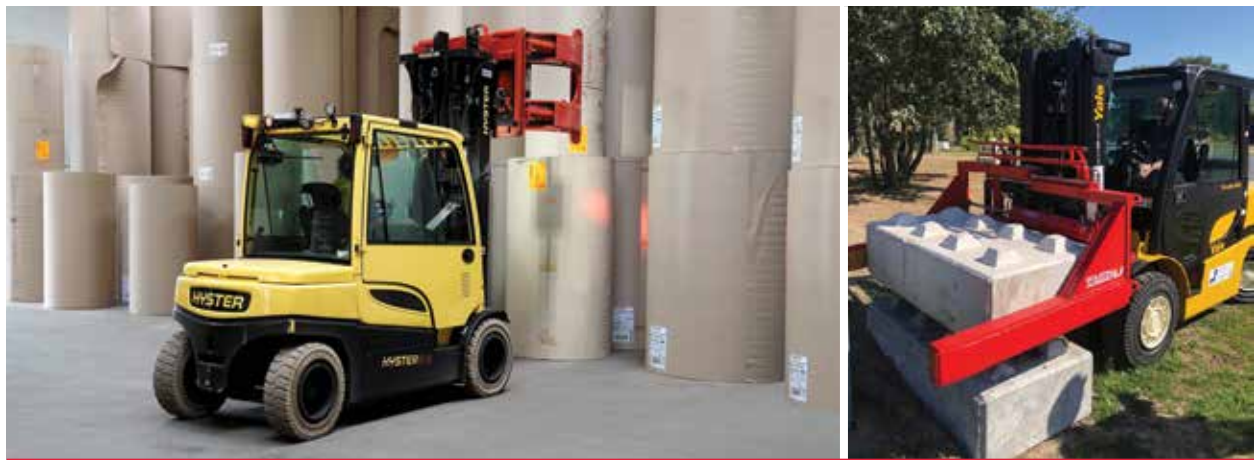
Hyster-Yale's leadership in the attachments business core strategy is synergistic to its other core strategy of providing customer- and industry-focused solutions. ▲ Left: A Bolzoni® paper roll clamp on a Hyster J5.5XN electric lift truck moves paper rolls at a European paper facility. ▲ Right: A Bolzoni block clamp, attached to a Yale® Veracitor® 40VX premium internal-combustion engine lift truck moves cement blocks at an outdoor location.
