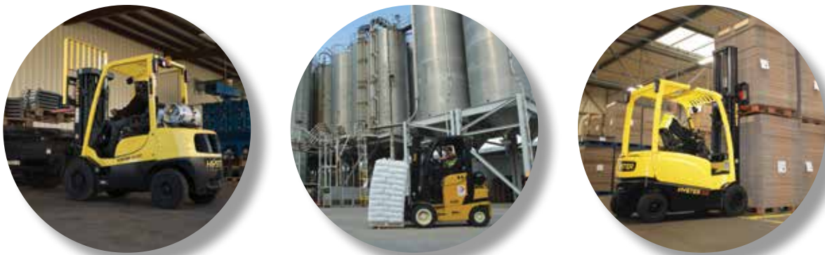
Hyster-Yale offers a full range of products and solutions for a variety of industry applications. ▲ Left: A Hyster® 60XT, with a lifting capacity of 6,000 pounds, moves steel plates in a steel manufacturing facility. ▲ Middle: A Yale® 2.5VX premium Veracitor lift truck moves a pallet of materials at a chemical plant. ▲ Right: A Hyster® J50, with a 5,000-pound capacity, moves cardboard at a paper and packaging facility.
