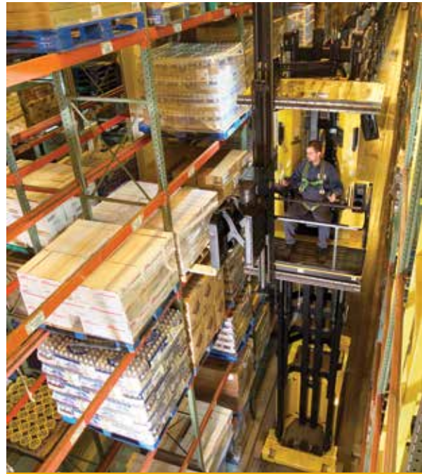
A Yale® NTA030 Turret truck is used in very narrow aisle retail warehouse applications.
