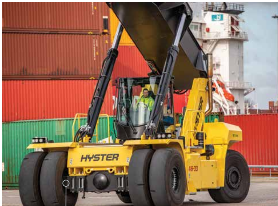
A Hyster® ReachStacker 46-33, shown here with the new enhanced ergonomic cab, is sturdy enough to move and stack heavy containers weighing up to 46,000 lbs. in port applications.
