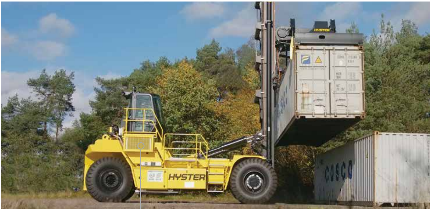
The hydrogen fuel cell radiator is clearly on display on the new 52-ton capacity Hyster® laden container handling electric truck currently located at the Company's testing facility in Weeze, Germany. This truck, powered by a hybrid system that utilizes both a lithium-ion battery and fuel-cell engine, is awaiting shipment to the Port of Los Angeles to begin its testing phase.
