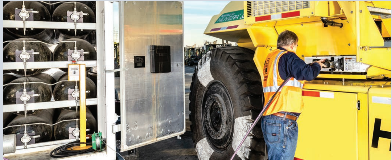
▲ The Hyster® 1150 CH, 52-ton electrified Big Truck, powered by two 45kW Nuvera® hydrogen fuel cells, is seen here refueling during operations at the Port of Los Angeles, California.
