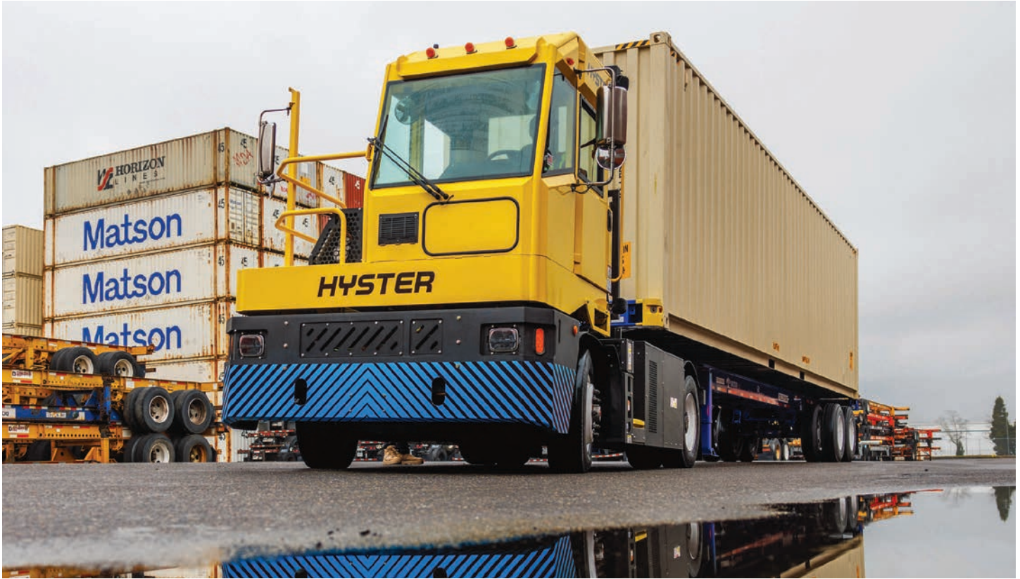
A Hyster® electric Terminal Tractor, powered by integrated lithium-ion batteries, transports a container in a shipyard.
