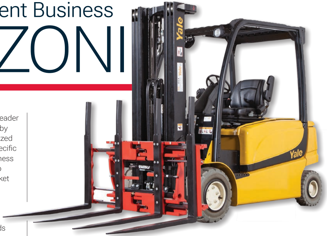
A Bolzoni Auramo® multiple pallet handler, which is often used for handling single or double loads of food or beverage products, is shown on an electric Yale® lift truck.
